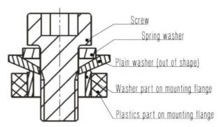
6.3.8 Please avoid grease and other foreign matter in the terminal please use the connecting wire with a cross section area  $\geq 300 \text{ mm}^2$ , or they may cause overheating to the terminal part.
