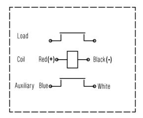
Load non-polarity; Auxiliary contacts have no polarity; coil has polarity
