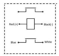
The load is non-polar, the coil is polar
